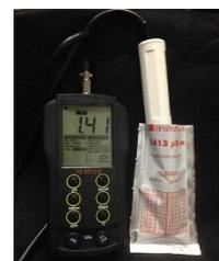
Photo 4. Calibrate the EC of your meter, noting the difference in units between the display of the EC meter and the labeled calibration solution.
