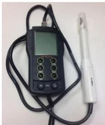
Photo 1. The Hanna Instruments HI 9313-6 meter that I will be using for demonstration purposes.
