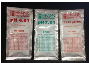
Photo 2. The standard solutions that match the meter I am using.
