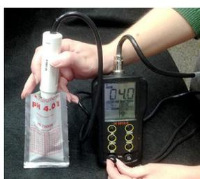
Photo 3. Calibrate your meter by turning the dial with the standard solution: 4.01 pH shown here.
